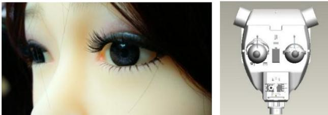
Figure-8: Eye module assembly
