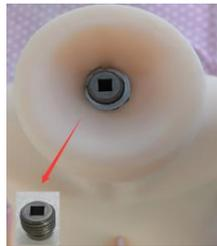
**Fig-15-1: Installation diagram for neck bolt(Third generation)**
